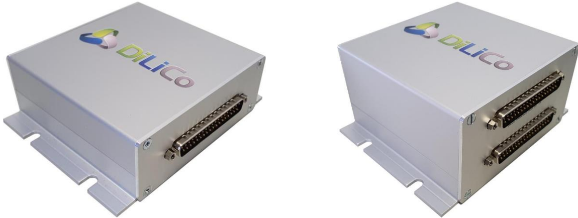
Figure 1: DiLiCo cell voltage 36 with 37-pin D-Sub connector for connecting 36 cells (130 x 110 x 40 mm 3 ) on the left and DiLiCo cell voltage 72 for connecting 72 cells (130 x 110 x 60 mm 3 ).
